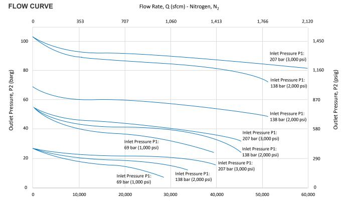
Flow Rate, Q (slpm) - Nitrogen, N<sup>2</sup>
